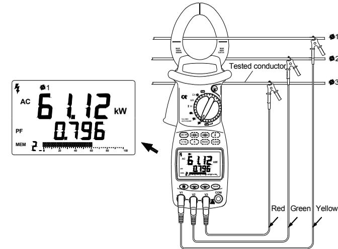
( Figure 17.Power Measurements Of Three-Phase Three-Wire)
